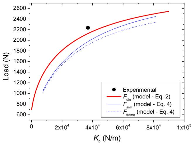
Figure 13 – Measured data and analytic models results for the loads as a function of suspension stiffness ( $K_2$ ) for  $h = 0.20$  m
