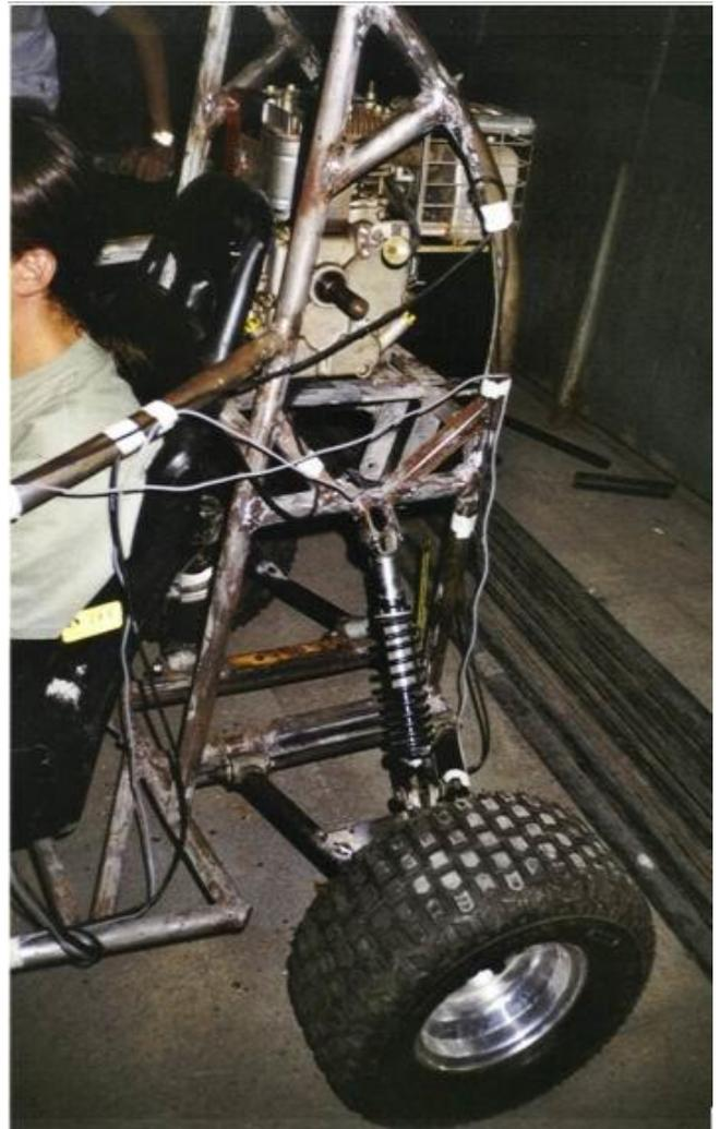
Figure 4 – Instrumentation of Mini-Baja rear suspension.
