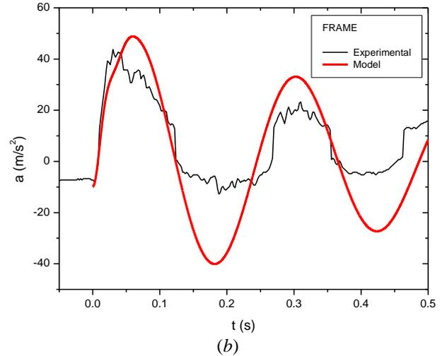
Figure 10 – Measured data and analytic model results for the rear suspension arm (a) and frame (b) for  $h = 0.20$  m.
