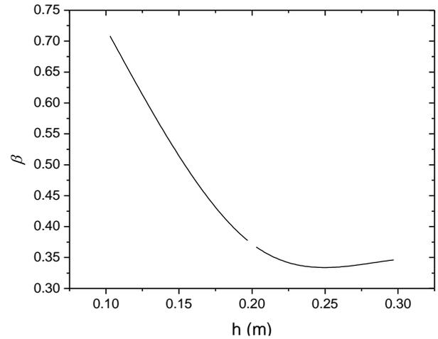
Figure 8 – Transmissibility factor  $\beta$  for several loading conditions.
