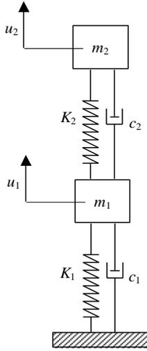
Figure 9 – A simple two-degree of freedom model for the rear suspension.
