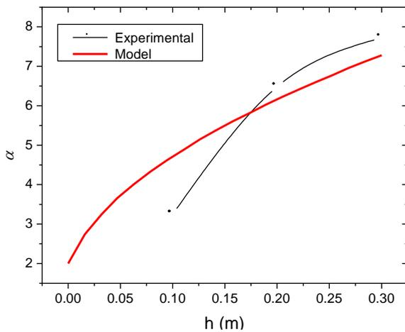
Figure 7 – Amplification factor  $\alpha$  for several dropping heights.
