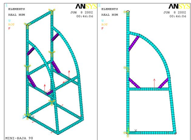
Figure 2 – Numerical analysis of the rear suspension. Finite element mesh with the applied loads and boundary conditions
