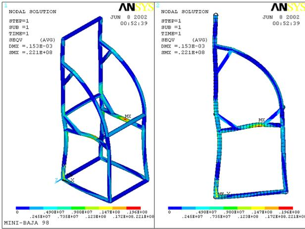
Figure 3 – Numerical analysis of the rear suspension. von Mises equivalent stress distribution.
